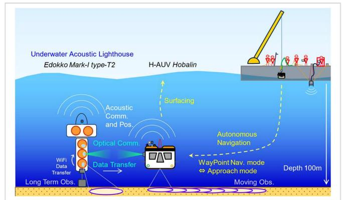
Fig. 1. Concept of the cooperative observation by Lander and H-AUV.
