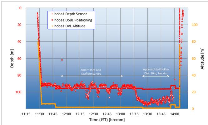
Fig. 4. -AUV *Hobalin* Depth and Altitude on May 29.
