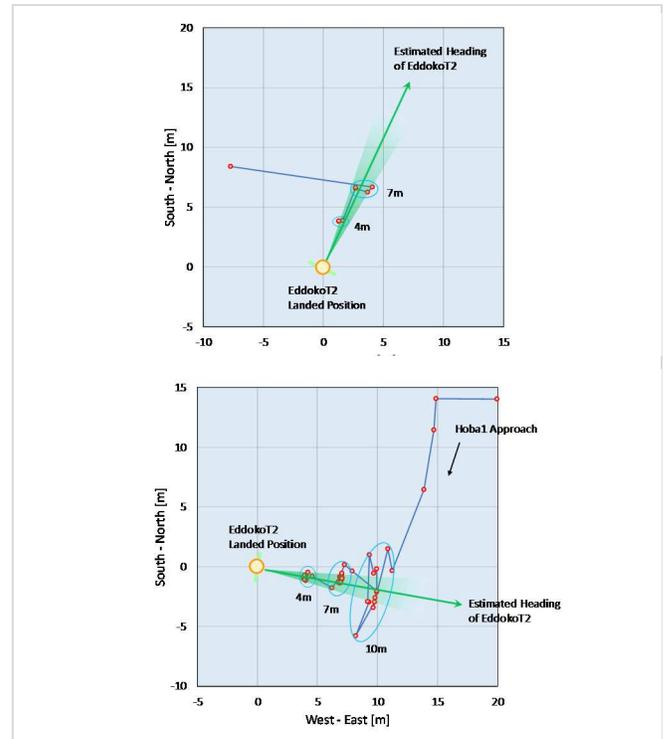
Fig. 6. USBL Positioning from *Edokko Mark-I* to *Hobalin* (Up: May 29, Down: May 30).
