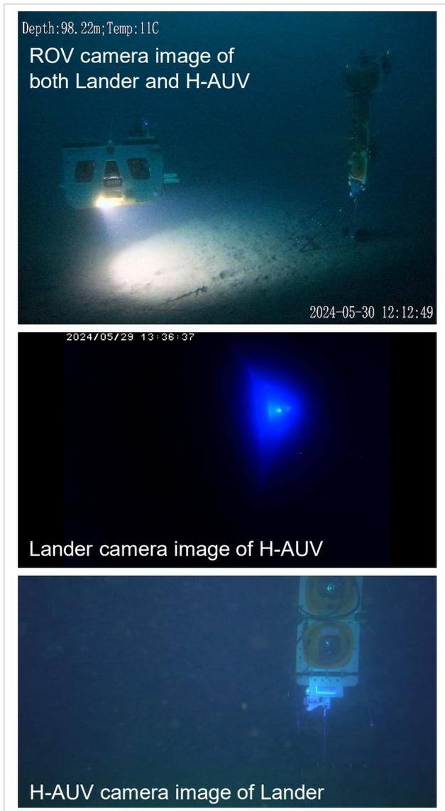
Fig. 7. Image samples near seafloor on May 29 and 30 (Top:ROV camera view, Middle: *Edokko Mark-I* camera view, Bottom: *Hobalin* camera view).
