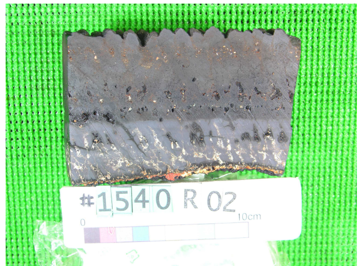
Fig. 1. Picture of Mn-crust sample (thickness = 85mm)
