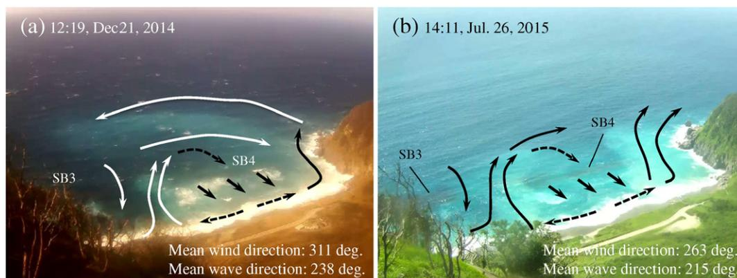
**Fig. 6.** Snapshot of nearshore currents taken by the webcam at 12:19 on December 21, 2014 (a) and at 14:11 on July 26, 2015 (b) visualized by the contrast in color of turbid beach waters and clear offshore waters and its temporal evolution (solid arrows). Broken arrows are deduced currents. 15-min animations made from the images taken every 5 s are also available online in the electronic version of this article (Appendix B).
